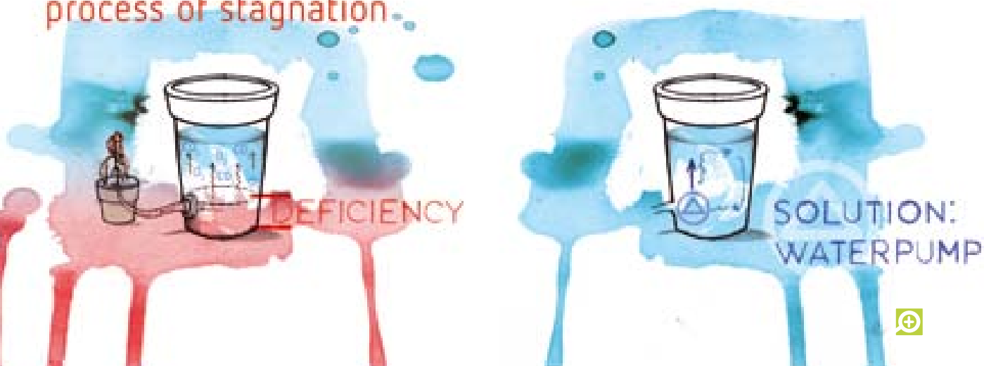
Figure 2: When the water in the nutrient holding tank is left still, the dissolved gases begin to leave the water by rising through the column of water so that there is less dissolved gas at the lower levels, with more towards the top.
